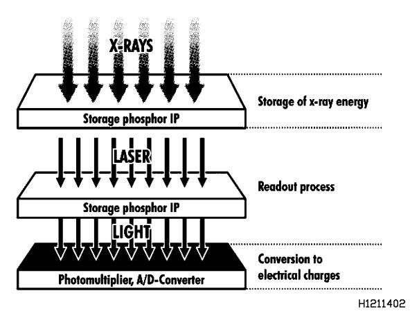
Figure 6-74. Example of Computed Radiography
