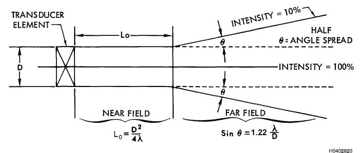
Figure 5-8. Schematic Presentation of Sound Beam
