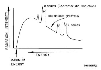
Figure 6-8. Typical X-ray Spectrum
