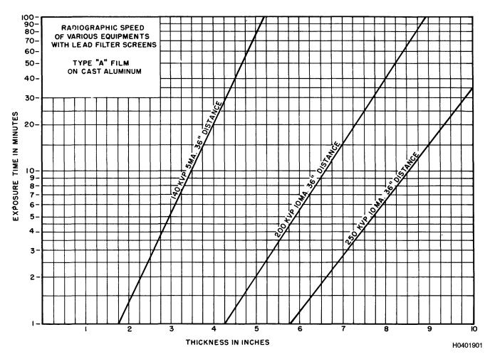
Figure 6-35. Typical Technique Constant-Density Chart
