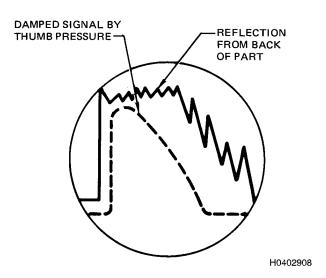
Figure 5-70. Damping Technique
