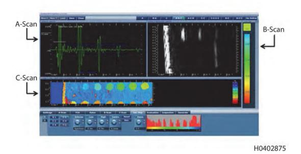
Figure 5-41. A-Scan, B-Scan and C-Scan Presentation Examples
