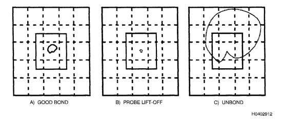
Figure 5-74. Pitch/Catch Swept-Frequency Signal Patterns
