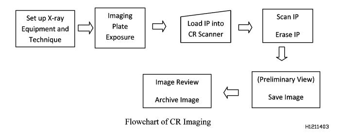
Figure 6-75. Flowchart of CR Imaging
