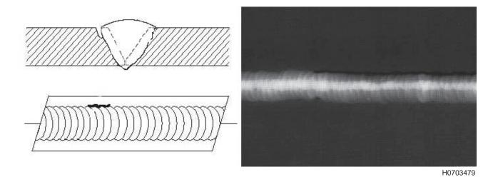
Figure 6-61. External Undercutting
