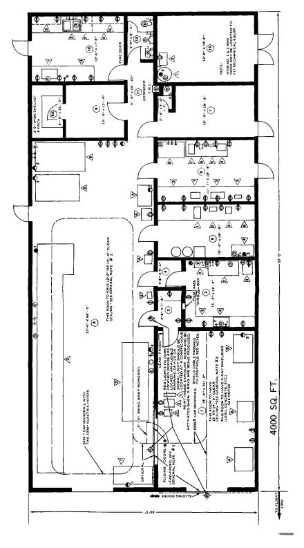
Figure 1-2. Typical Nondestructive Inspection Facility
