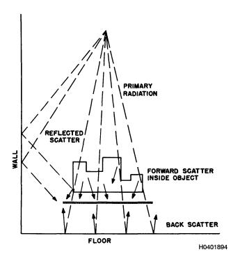
Figure 6-28. Sources of Scatter Radiation
