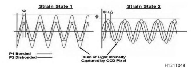
Figure 7-2. Coherent Single Frequency Light
