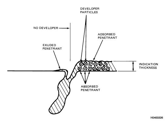
Figure 2-8. The Effects of a Developer
