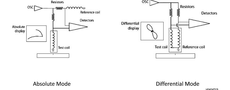
Figure 4-27. Example of Absolute and Differential Mode
