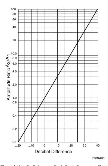
Figure 5-18. Decibel-to-Amplitude-Ratio Conversion Chart
