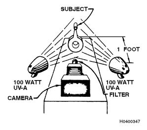
Figure 2-32. Location of Camera and Lights for Photographing Fluorescent Indications
