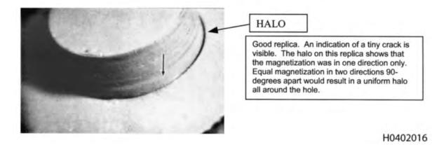
Figure 3-35. Magnetic Rubber Replica With Good Indication
