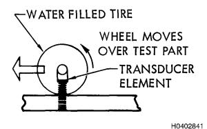
Figure 5-26. Wheel Transducer
