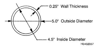
Figure 3-72. Calculating Effective Diameter
