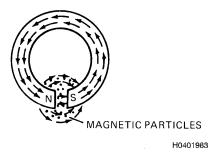
Figure 3-2. Horseshoe Magnet With Poles Close Together
