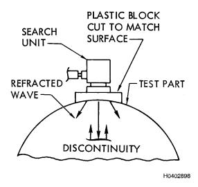
Figure 5-61. Convex Sound Entry Surface
