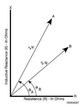
Figure 4-12. Vector Representation of Impedance
