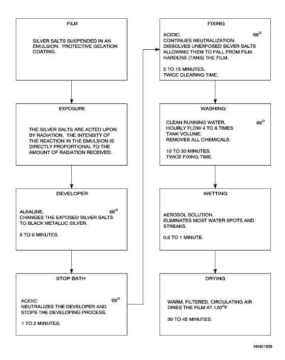
Figure 6-42. Manual Film Processing
